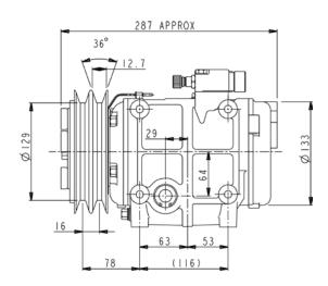
This TM type fixed displacement swash plate piston type compressor is adaptable to any type of field application, from small engine to heavy duty, including bus applications.
