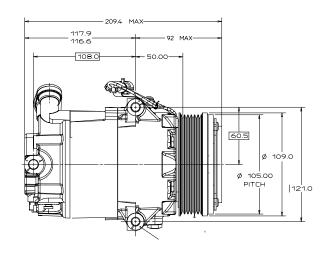
The next generation of variable displacement piston compressor technology, Delphi's Compact Variable Compressors (CVC), are based on a swash plate simple harmonic motion mechanism. The enhanced mechanism performance makes the CVC adaptable to both pneumatic and electronic controls. Refrigerant R134a.
