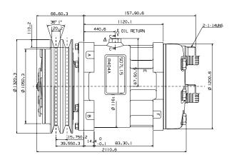
This compressor is equipped with 7 pistons, and it has (154 cm³) displacement/revolution. The reliability of this compressor is among the highest in the market. The compressor body is equipped with 8 "ears"; this feature, along with the mounting angle (+/-90°), allows for using the best mounting options. This SD7L15 compressor, is the version for R404a. The compressors are available with Rotalock ports (1" 14 UNS).
